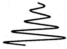
FIGURE 4-9 Spatial variation of the perturbed density in a plasma wave, as indicated by an interferometer, which multiplies the instantaneous density signals from two probes and takes the time average. The interferometer is tuned to the wave frequency, which varies with the density. The apparent damping at low densities is caused by noise in the plasma. [From Barrett, Jones, and Franklin, loc. cit. ]
